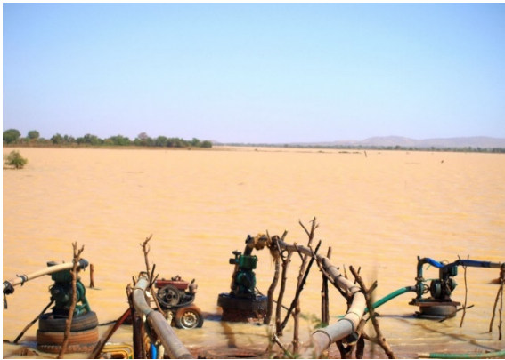
Figure 11: The pumping of water out of reservoirs for agricultural use (Source: A. Melcher)
